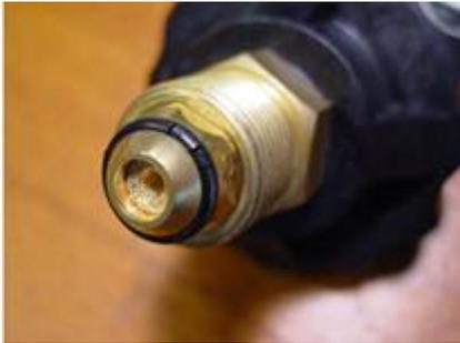
*Cracked deformed cylinder nipple o-ring.*
